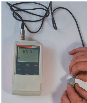
Coating thickness measurements
